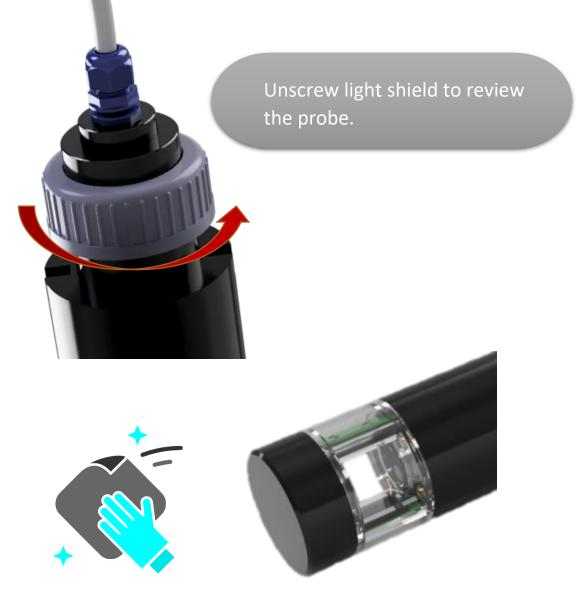
Clean the optical components around the probe. That is, the clear plastic and glass windows with a damp cloth and then dry
